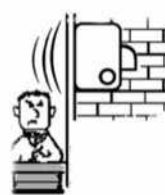
Hand dryer transmits noise by vibrating the wall.
