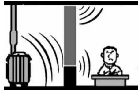
Even small cracks and holes leak a large amount of noise.
