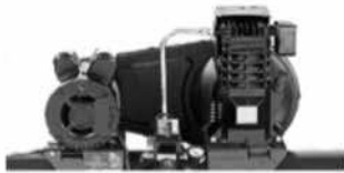
Solid guard will radiate vibrations and sound.
