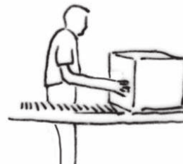
Use conveyors to move materials
